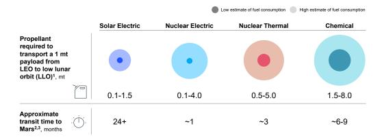
Entirety of spacecraft considered payload except for engine, power system, and propellant; assumes lsp of 1,000-10,000s for electric propulsion, 500-1,500s for nuclear thermal (NTP), and 250-450s for chemical and engine masses of 0.05-0.2 mt for solar electric (SEP), 0.7-2.0 mt for nuclear electric (NEP), 0.7-3.0 mt for NTP, and 0.1-1 mt for chemical; assumes full propellant mass is consumed by end of maneuver
